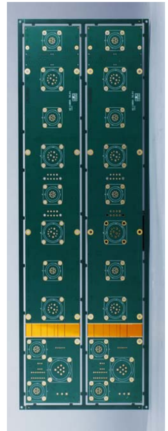
Flex and rigid flex boards are panelized for efficient and cost-effective manufacturing.
